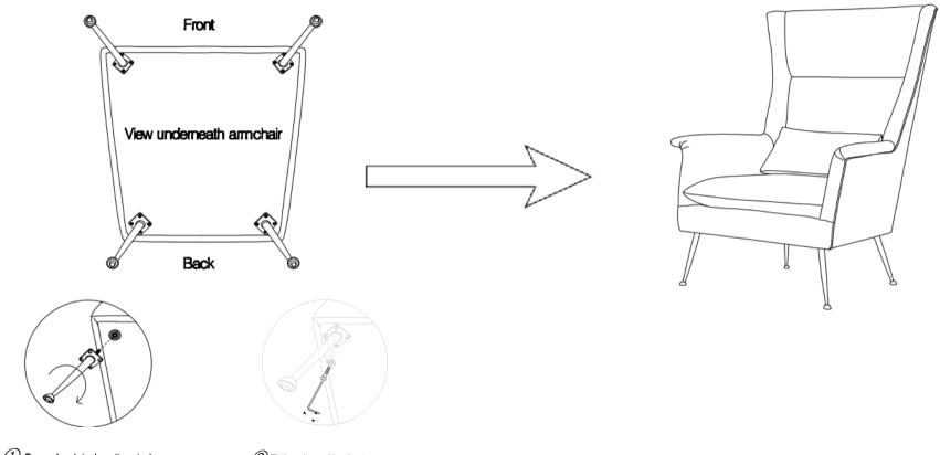
Screw leg into locating hole as diagram(4 holes located in each comer of base of chair)
