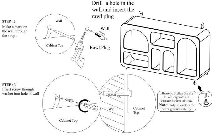
NOTE: Wall Fixings are not supplied with this product as different wall materials require different types of fixing devices (such as Rawl plugs on brick work) You must use fixing devices suitable for the type of wall you intend to mount this product to. Please ensure that the head of any screw used has a diameter greater than the diameter of the mounting hole on the product and that the fixing is safe and secure before use.
