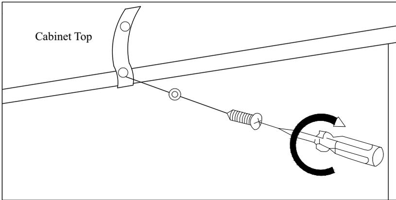
Drill a hole in the wall and insert the rawl plug .
