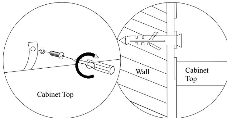
**NOTE:** Wall Fixings are not supplied with this product as different wall materials require different types of fixing devices (such as Rawl plugs on brick work) You must use fixing devices suitable for the type of wall you intend to mount this product to. Please ensure that the head of any screw used has a diameter greater than the diameter of the mounting hole on the product and that the fixing is safe and secure before use.
