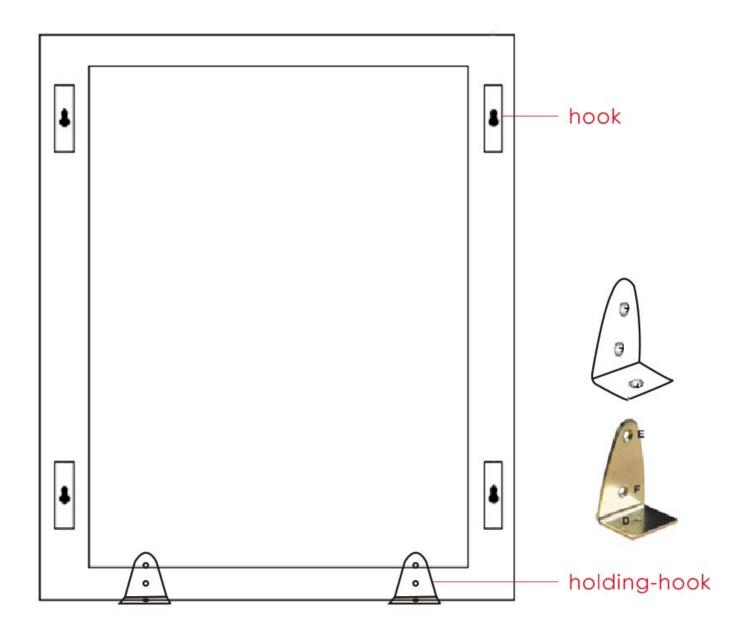
In order to keep more stability and safety, please install the holding hooks on the bottom side!!
